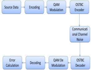
Fig: 1 Block diagram of the communication system
