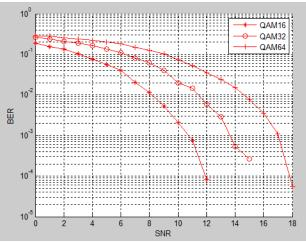
Fig: 3 BER curve for 4 antenna OSTBC encoding with zero forcing equalization
